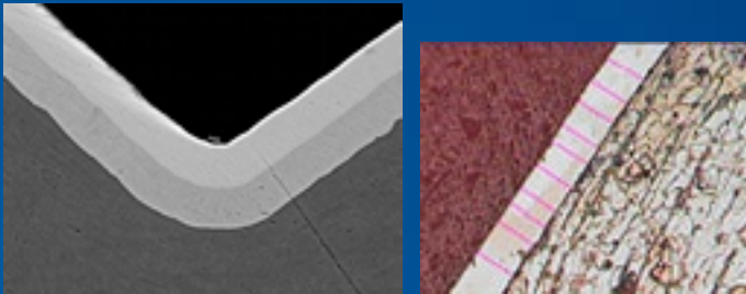
Cross section analysis on chrome plating coating
