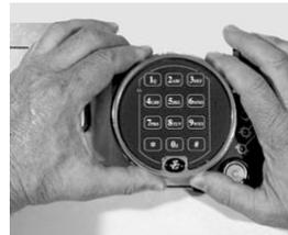
12. Place the keypad over the base. Make sure the keypad cable is clear of the pad's two spring clips as you push the keypad firmly onto the base. It should snap into place. If you need to remove the keypad, pull the bottom (area nearest the S&G logo) away from the mounting base first. Never allow the keypad to hang by the attached cable. The installation is complete, but do not close the safe door until successfully completing the following lock test.
